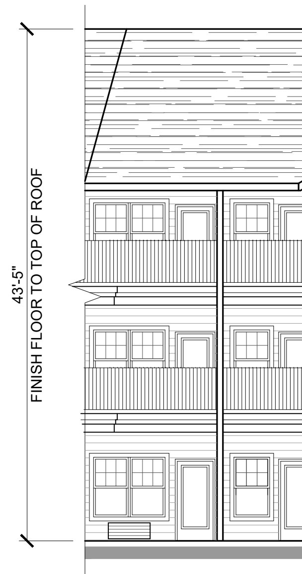
3-STORY FINISH FLOOR TO TOP OF ROOF
